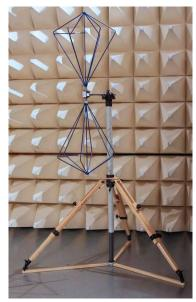
VBA 6106A vertical onto tripod BTP 6020A
