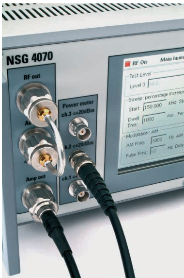
NSG 4070 front panel with RF ports
