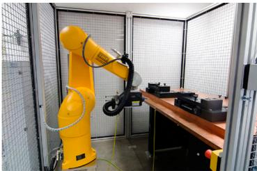
Complete system solution with 30 kV ESD simulator for robotic applications.
