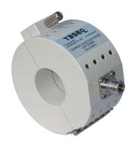
The CIP 9136 probe has been manufactured to drawings and specifications laid down by QinetiQ. It meets the requirements for HIRF testing where conventional ferrite core material cannot handle the higher powers required (up to 1000 W), without changing characteristics when heated. Whilst having been initially designed to meet the specific requirements of Aircraft Testing from 10 kHz to 50 MHz, the CIP 9136's unique non-ferrite core allows wide band performance from 10 kHz - 400 MHz, and above.
