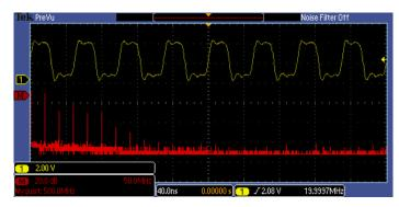
Analyze - FFT analysis of a pulsed signal. A comprehensive set of integrated analysis tools speeds verification of your design's performance.
