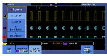
Capture – Triggering on a specific transmit data packet going across an RS-232 bus. A complete set of triggers, including triggers for specific serial packet content, ensures you quickly capture your event of interest.
