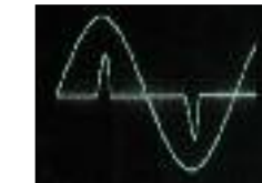
Same conditions as above with programmable Z^{\circ} engaged. THD=0.25%
