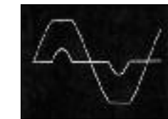
Oscilloscope of voltage and current waveform at load due to distribution losses. THD=6.6%
