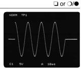
Output ON/OFF Phase Setting Output on phase: 90 deg. Output off phase: 0 deg
