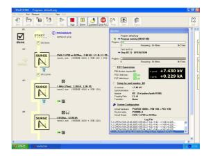
System configuration is an extension of the plug & play philosophy. Hardware attached to the system bus is auto-detected. Individual test instrument specifications are displayed and made available. Individual test and program execution times are displayed giving a detailed preview of the complete process.
