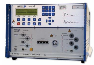
The modular concept is built around a PC based host controller (the PSURGE 8000 Controller) with physically and functionally independent modules for impulses (PIM #X), coupling/decoupling (PCD #X). The system uses distributed intelligence, and each module has its own application-specific program, runs internal routines and communicates with the host controller. System modules are automatically detected by the host controller, providing true Plug & Play functionality.
