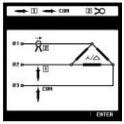
• **New!** On screen graphics show you how to set up 3-phase power measurements
