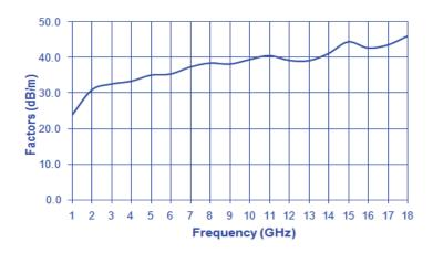
$Field\ strength\ (dBV/m) = Output\ measured\ (dBV) + Antenna\ Factor\ (dB/m)$
