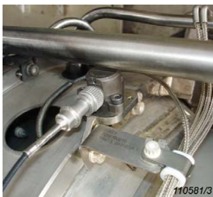
Fig. 3 Charge Accelerometer Type 8324 shown fitted to engine bracket
