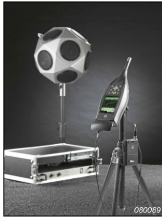
Fig. 10 Optional wireless systems are available to control the sound source for airborne (left) and impact (right) sound insulation measurements
