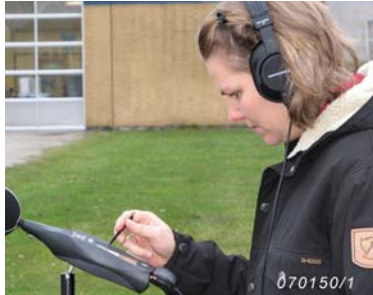
Fig. 14 Performing an outdoor tone assessment measurement
