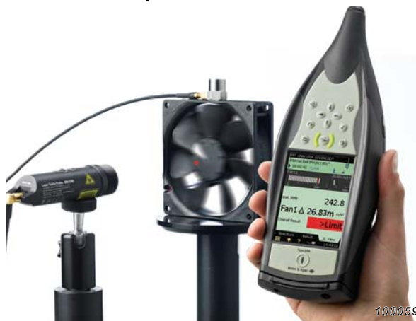
Fig. 10 Type 2250-H-D01 with Laser Tacho Probe Type 2981 in product vibration testing
