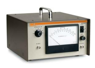
C63.2 specifications for single frequency RFI instruments and is compatible with the NM-17/27A and NM-25T for all pulse repetition rates above 50 pulses per second. The instrument is hand portable, withstands rough field use and has low (5 watt) power consumption.
