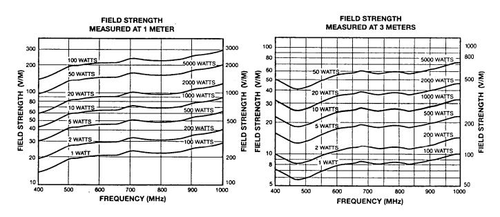
Field strengths have been measured in free-space conditions. Individual shielded rooms, amplifiers, and test-system conditions will influence performance. Field strength also varies with frequency and position of antenna and EUT in non-anechoic testing environments.
