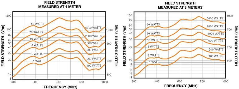
Field strengths have been measured in free-space conditions. Individual shielded rooms, amplifiers, and test-system conditions will influence performance. Field strength also varies with frequency and position of antenna and EUT in non-anechoic testing environments.
