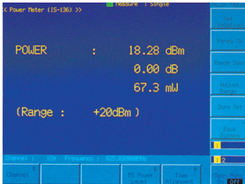
Example of power measurement
