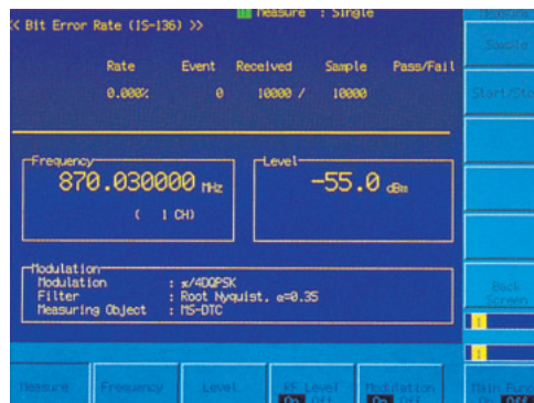
Bit error rate measurement (IS-136A)
