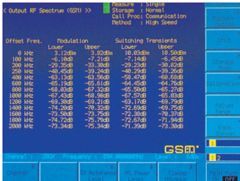
Output RF spectrum measurement (GSM)
