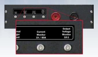
Scaled Voltage and Current ports provide the data needed to complete Requirements R1, R2, R3, R4 and R5 of the ATIS standard.
