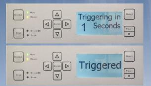
The 4301 provides a built-in Trigger function for triggering the DC pulse during testing.
