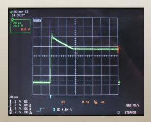
The 4301 can output transient voltages of 50-100V in less than 2µS, or 5-100V in less than 5µS (shown). It can reproduce either the combined waveform/ single measurement or the multiple waveform/ multiple measurement methods described in the ATIS standard.
